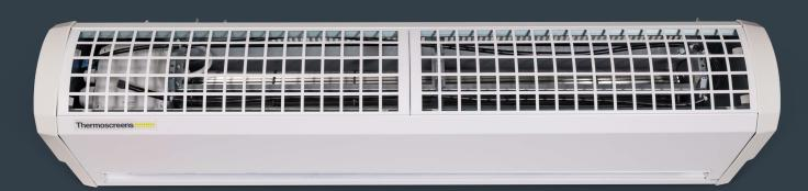
Designed and engineered to maintain climate separation in cold stores with temperatures as low as -25 degrees Celsius. The Slimline CS Series has advanced EC motor technology, so not only does it keep the cold store cold, but also keeps energy consumption to a minimum. The unit benefits from built-in frost protection to ensure unhindered access for goods. Specifically designed for applications where there's limited headspace above the door, this series is compact and cost-effective.
