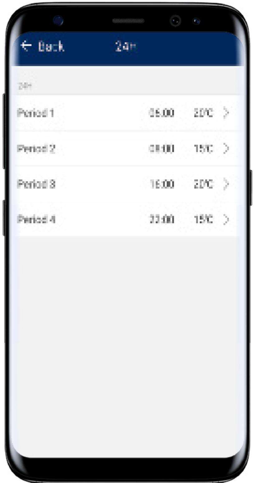
**24 Hours** – This allows you to change the set temperature point for a 24 hour cycle.
